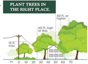
Plant shrubs at least 10 feet from the transformer door and 4 feet from the sides. If your property has underground lines, contact 811 before you begin any project requiring digging. Additionally, if you spot an overgrown tree or branch dangerously close to overhead lines, please get in touch with us at 1-800-635-4145.
